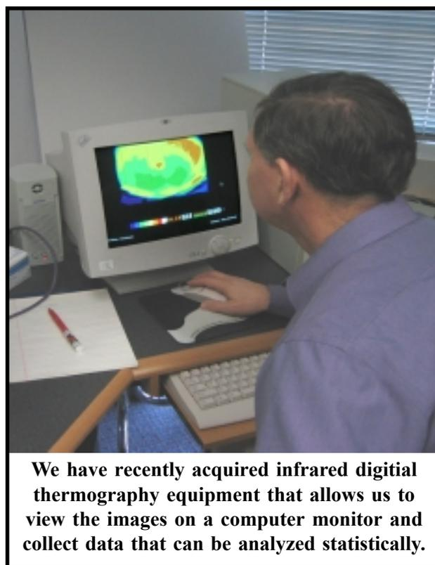
**We have recently acquired infrared digital thermography equipment that allows us to view the images on a computer monitor and collect data that can be analyzed statistically.**
